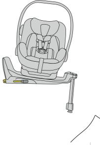
To rotate the car seat, pull or push lever A and turn the seat with one hand in the desired direction.
