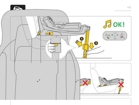
Press the foot extension button (a) and extend the leg until the foot is firmly placed on the vehicle's floor. During proper installation, the foot's light on the display will change from red to green.
