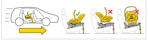
Place the car seat in the base. To do this, insert the car seat from side (a) into the base's hooks, and then push the car seat into place (b) in the base. After properly inserting the car seat into the base, a green light will appear on the display on the right side.
