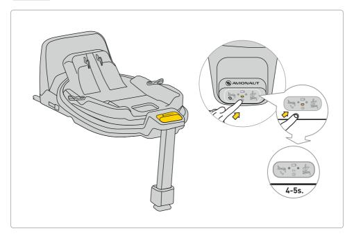
To mute the sound, press the display button for 4-5 seconds. The display will still show the correct/incorrect seatbelt and base attachment, but the sound will be muted.
