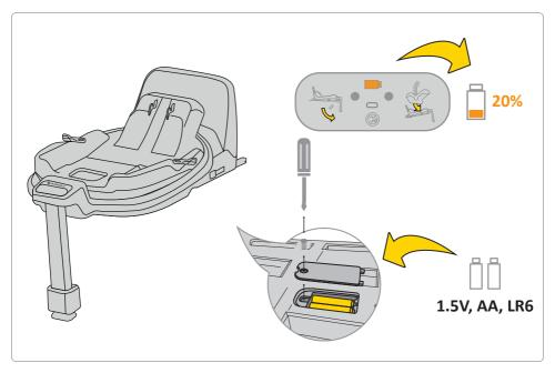
If the battery indicator on the display is orange, it needs to be replaced. To do this, remove the cover at the base and take out the batteries.
