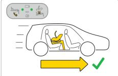
Before setting out on a journey with your child, perform a test of the base's electronic system. After properly securing the car seat and mounting the leg, two green dots should appear on the display.
