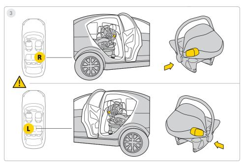
Always mount the bumper on the car seat towards the vehicle's door side.
