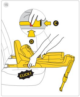
To insert the leg, press the button  $\triangle$  and insert leg  $\bigcirc$  to its original position, and then fold it to save space.
