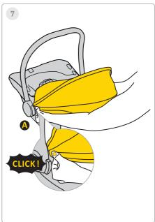
To attach the canopy to the car seat, mount frame 1 and press it against the canopy mount.
