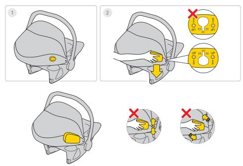
The car seat has a bumper mounting on both sides.
