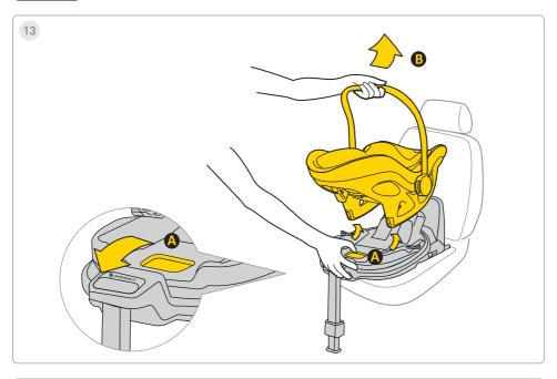
To remove the car seat from the base, pull the release handle a and gently tilt the seat forward while lifting it up by the handle b.
